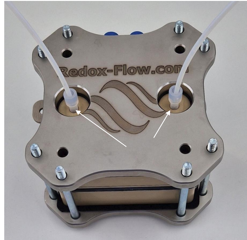
B. Tube fittings are mounted in cell
