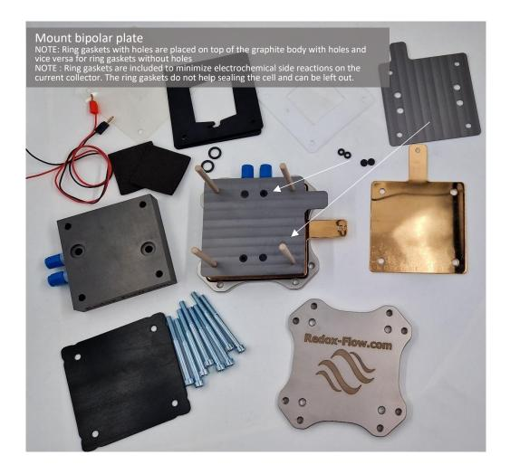
End of bipolar plate assembly. From here the assembly is the same for both assemblies.
