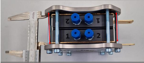
Quality of the cross tightened is checked by measuring the distance between the endplates at all four corners. The distance should not vary more than 0.1-0.2mm. NOTE: Step 1 and 2 can be performed iteratively.
