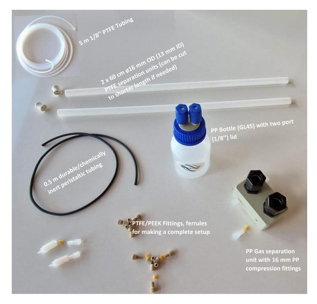
The whole setup comes unassembled and the 1/8" tubing in one piece, thereby giving larger flexibility.
